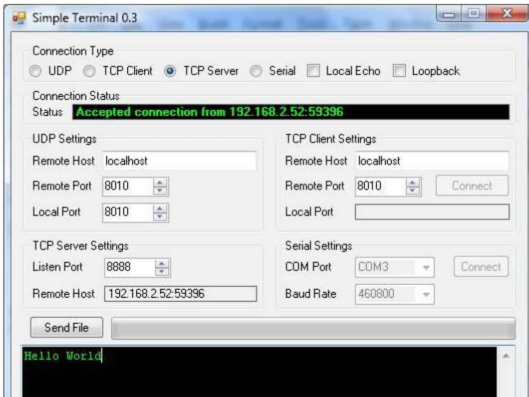
Screen 18: Simple Terminal TCP Server Setup
