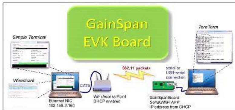
Figure 1 Serial to Wi-Fi Bridge Test Setup
