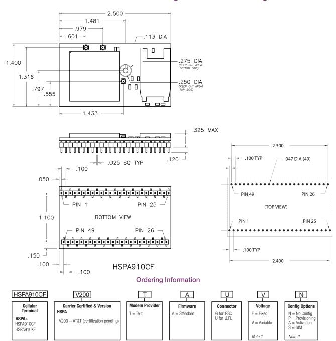
Example: Part Number – HSPA910CFV200TAUVN = HSPA+ Cellular Plug-In Terminal; AT&T Certified (pending); Telit Modem; Standard Firmware with a U.FL Connector and a Variable Voltage with no configuration options.
