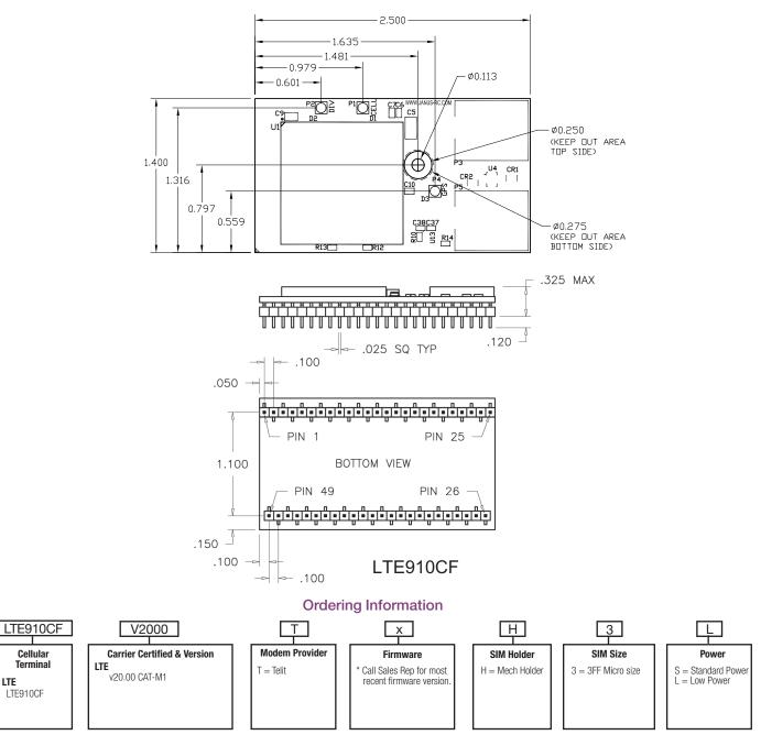
Example: Part Number – LTE910CFV2000TxH3L = LTE Cellular Embedded Modem; Telit Modem; Current Firmware; Mech SIM Holder; SIM Size Card 3FF Micro; Low Power.
