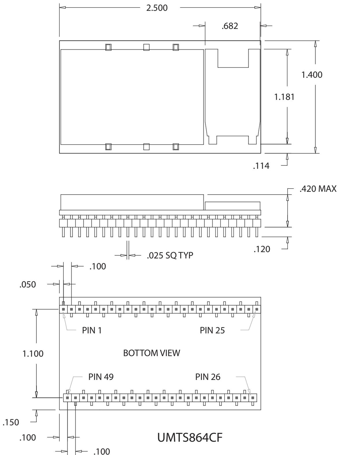
**Figure 17 UMTS864CF Mechanical Dimensions**
