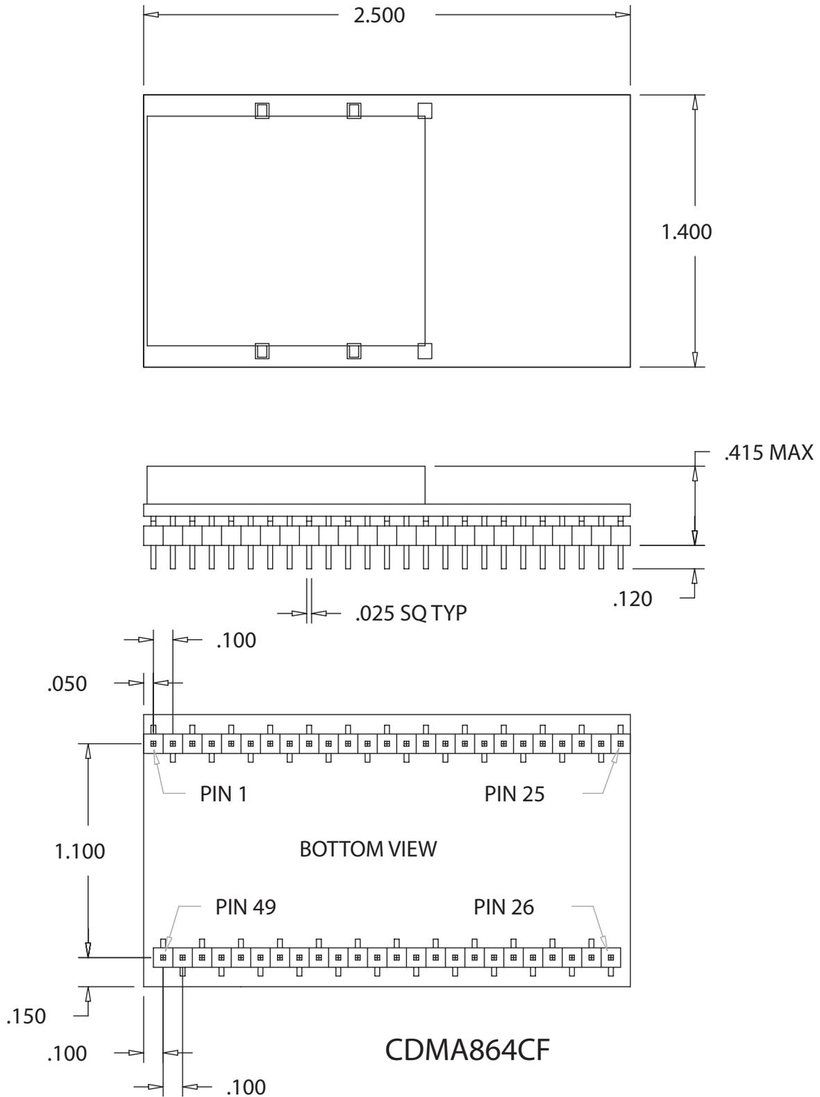
Figure 16 CDMA864CF Mechanical Dimensions
