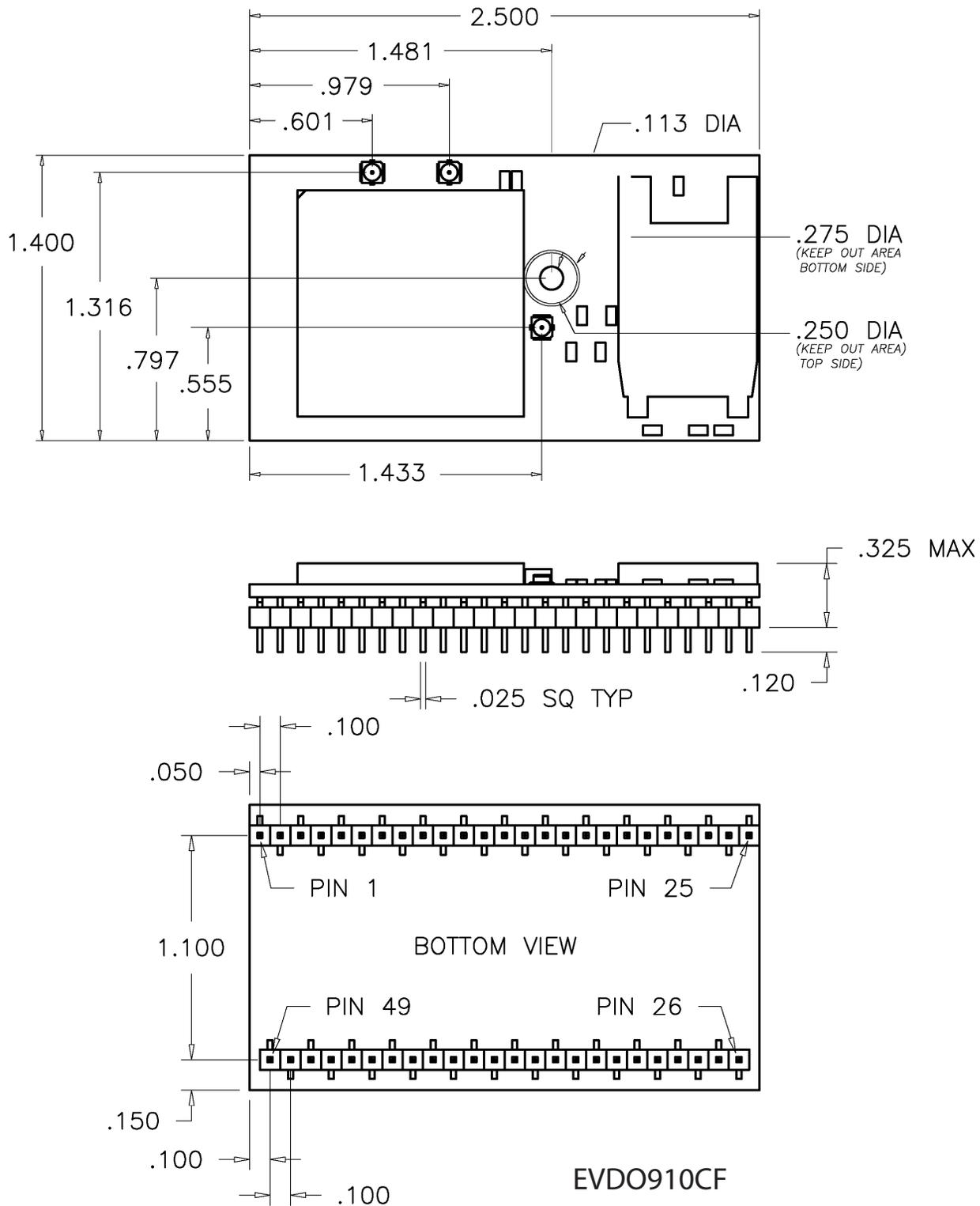
Figure 18 EVDO910CF Mechanical Dimensions
