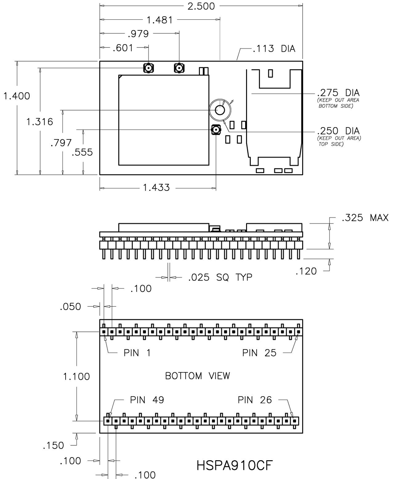
**Figure 18 HSPA910CF Mechanical Dimensions**
