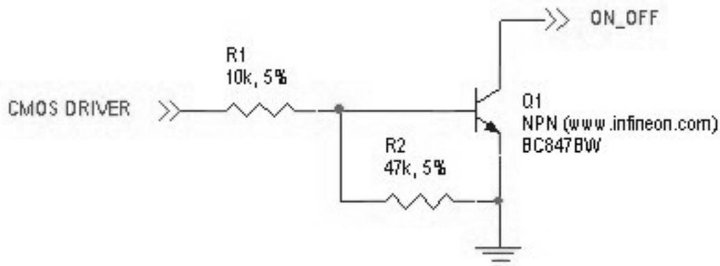
Figure 12 On / Off Pin Diagram
