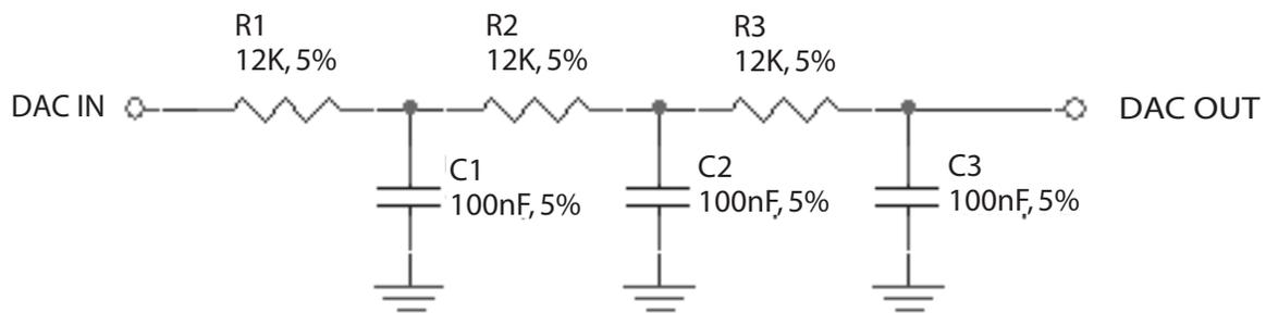
Figure 14 Required DAC Filter
