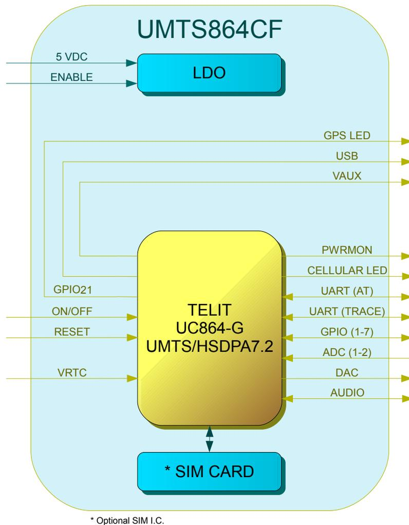
Figure 3 UMTS Block Diagram
