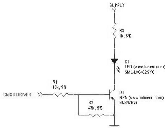
Figure 13 LED Indicators Diagram
