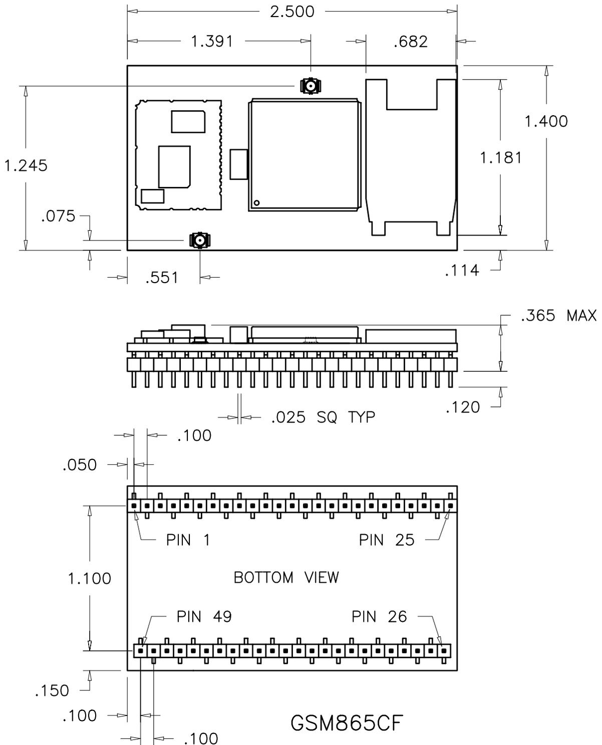
Figure 15 GSM865CF Mechanical Dimensions
