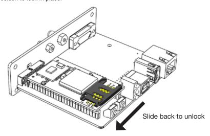
Step 5. Slide the back panel and 400AP board into the aluminum enclosure. Replace the four TX-10 screws and tighten them back on to enclosure.
