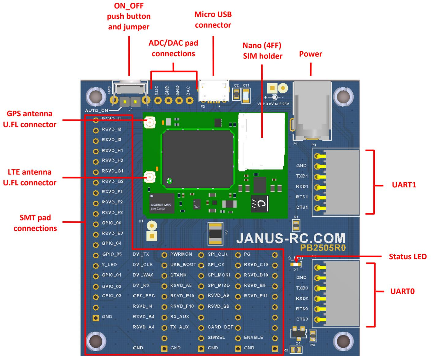
Figure 1: LTE310SMT Connections
