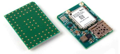
The LTE310SMT LGA Modem allows end users to assemble “end device” certified embedded cellular modems right onto application PCBs. No more hand assembly. No more modem pin connection issues in the field. Our CellBridge™ SMT units are designed to be placed during the primary pick & place assembly process, like all other primary BOM components.
