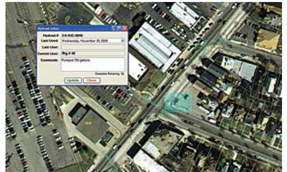
Once a truck has used a fire hydrant, that hydrant feature is flagged in the system.
