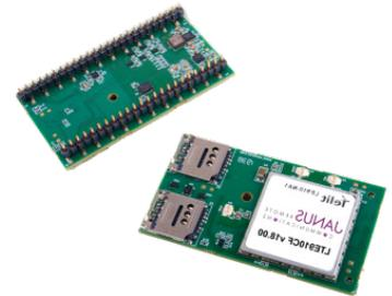
Easily integrated into any new or existing hardware applications via its standard 49-pin DIP configuration, the LTE910CF is a cost-effective solution for LTE IoT (Internet of Things) connectivity. Users can choose to mount the devices directly onto their PC Board or simply mount in a DIP socket or header. Their footprint compatibility with other Janus products removes the worry of obsolescence.
