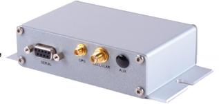
Incorporating carrier end device certified Common Footprint Embedded modems, the LTE910T3 provides a hardware solution with direct access to the cellular network of your choice. External connectors allow the customer to choose the precise antenna for their application needs.
