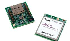
The full XF line shares the Industry Standard 20-pin connector footprint and is flexible in implementation - both into new product designs and with existing products.
