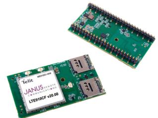
The **LTE910CF v20.00** CAT-M1/NB2 Cellular Modem uses the Telit ME910G1-WW as its cellular engine and has global PTCRB, AT&T, Verizon and RED certifications. The **LTE910CF v20.00** units operate in CAT-M1/NB2 LTE 4G and 2G bands. (See bands on our website)
