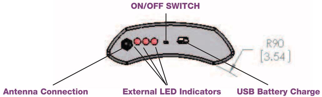
Figure 3 External Connections
