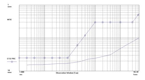
The graph below demonstrates the ability of the 125 Series Wi125 to continue to provide a GPS disciplined output frequency with the GPS aerial located completely inside a building (the degradation of MTIE performance is due to the effects of signal multi-path)
